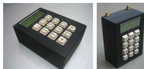
Figure 7 Prototype of the *box. Note the golden pigtail connectors on the top of the box to allow easy attachment of GSM and GPS antennas.
